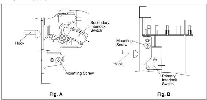
**NOTE**: A small gab may be acceptable if the microwave leakage does not exceed 4mW/cm<sup>2</sup>.
